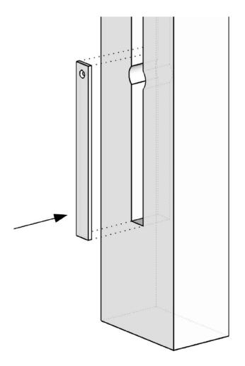
Install the bearing plates into the leg and the chop at the bottom of the mortises. They should slip into the mortise easily and rest on the end of the mortise and flatly on the bottom. Make sure you don't trap any wood shavings or chips behind the plate. The plate needs to be flat to the mortise bottom. Position the countersunk hole at the top, predrill, then drive the included wood screw to secure the plate.
